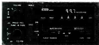
FIG. 2—THIS DELCO/BOSE cassette/receiver features automatic recognition of Dolby-B encoded tapes
